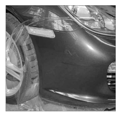
The film is applied as a wide sheet, covering the entire front bumper. Joe carefully sprayed a water and ammonia solution on the paint and adhesive side of the film, and then used a 3" wide rubber squeegee to squeeze the liquid and air bubbles from beneath the film. A razor cutter was used at body seams, with the excess peeled away.
